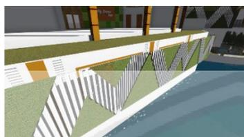
MEMBERI SECONDARY SKIN PADA BAGIAN YANG TERKENA INTENSITAS CAHAYA MATAHARI TINGGI, YAITU PADA BAGIAN TIMUR DAN BARAT. SECONDARY SKIN TERBUAT DARI ALUMUNIUM DAN VEGETASI SEHINGGA MASIH MEMUNGKINKAN ANGIN UNTUK MASUK KEDALAM BANGUNAN
